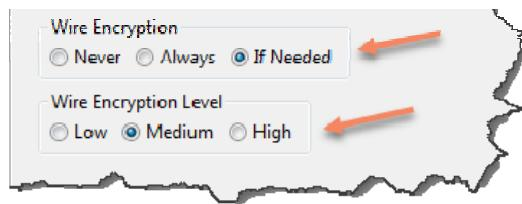
The default for *Wire Encryption* on both sides is “If Needed”, which means that encryption will NOT be used unless this setting is changed. If you set the server to “Always”, then every connection to that server will be encrypted. If you set a workstation to “Always”, then every connection from that client will be encrypted. The default for *Wire Encryption Level* is “Medium”, though we recommend changing this to “High” to use 128-bit encryption.
