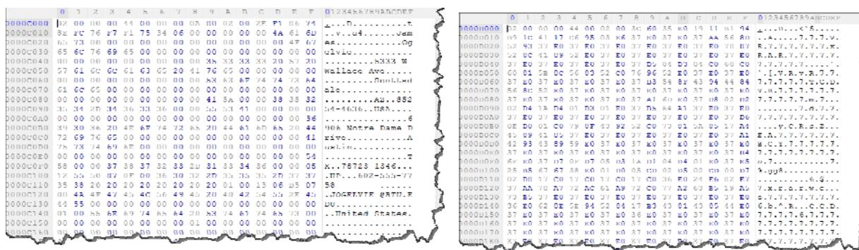
As you can see, file level encryption will prevent users from accessing your data by simply reading the data files directly. Because it is an undocumented encryption algorithm, this data is expected to be fairly secure, as well.
